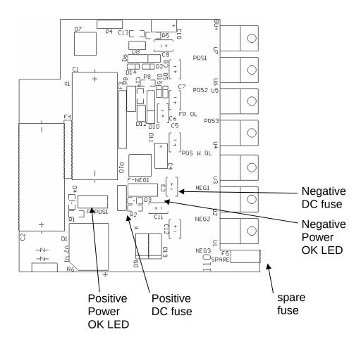
The spare fuse may be used to replace one of the other fuses, if required.
