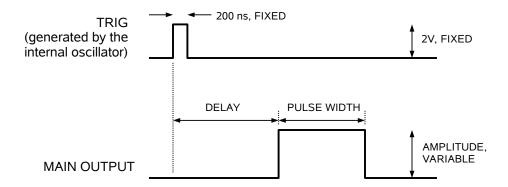
When triggered externally, the TRIG connector acts as an input. The delay controls do not function in this mode. This illustrated below:
