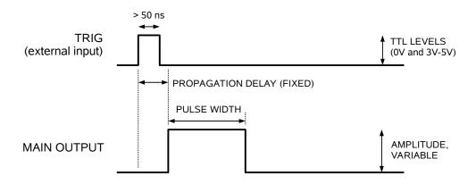
Units with the -ECL option require an ECL-level trigger, rather than a TTL-level trigger.
