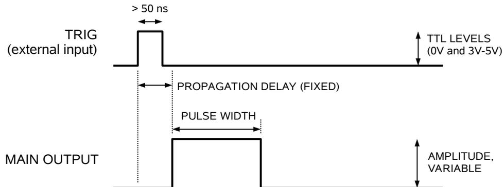
Units with the -ECL option require an ECL-level trigger, rather than a TTL-level trigger.
