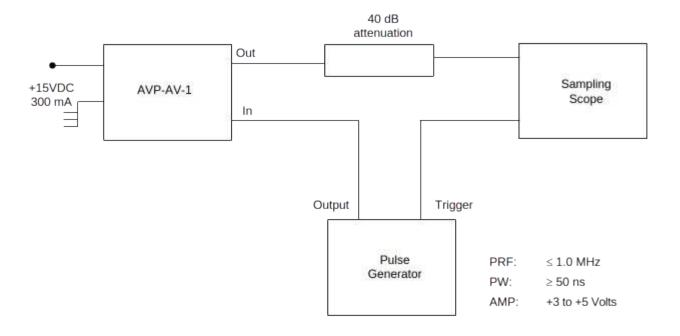
Power Line: +15 Volts / 0.3 Amps DC, shielded twisted pair, < 3 meters length
