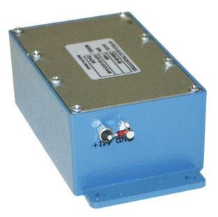
The +12V input terminal is protected with a Zener diode, which will fail as a short if an excessive positive voltage (> 15V), or a negative voltage, is applied to the terminal.
