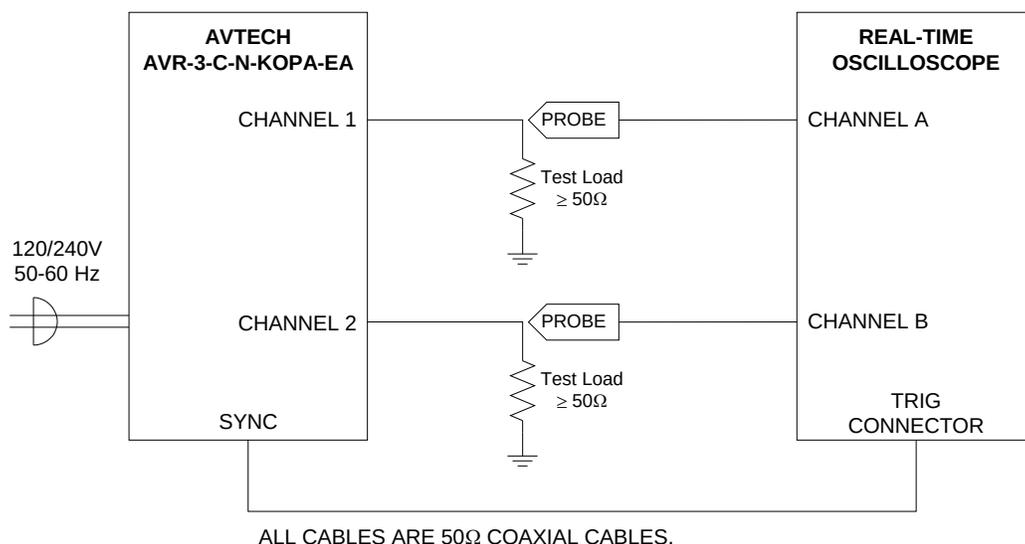
In this diagram, it is assumed that the rear-panel “AMP” switch is set to “INT”, in which case the amplitude of the two outputs is controlled by the single front-panel amplitude dial.
