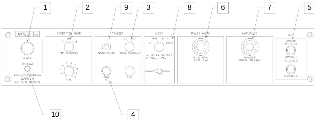
1. **POWER Switch.** The POWER push button switch applies AC prime power to the primaries of the transformer, turning the instrument on. The push button lamp (#382 type) is connected to the internal +15V DC supply.
