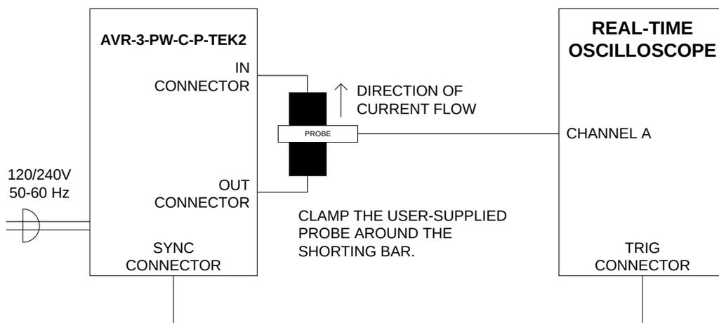
For other applications, the OUT terminal may be used to pulse a user-supplied 50 Ohm load, if desired. In this case, the shorting bar and the "IN" terminal are not used.
