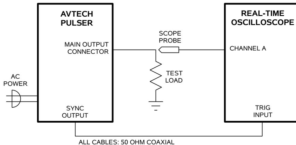
1. Connect a cable from the SYNC OUT connector to the TRIG input of an oscilloscope. Connect a 50W (or higher) 50Ω load to the OUT connector and place the scope probe across this load. The load resistor must have a voltage rating of at least 250V. The power dissipated in the resistor is given by
