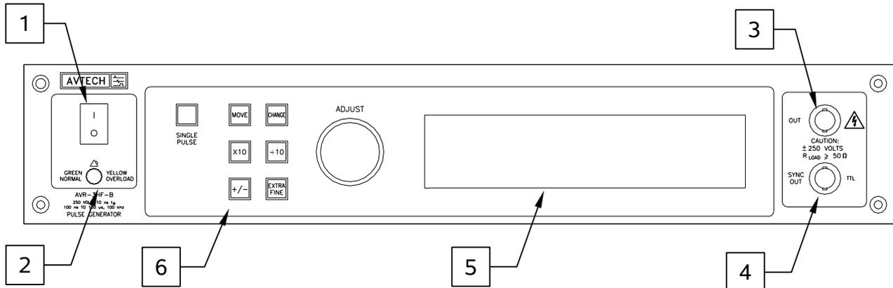
1. **POWER Switch.** This is the main power switch. When turning the instrument on, there is normally a delay of 10 seconds before anything is shown on the main display, as the internal operating system boots up.
