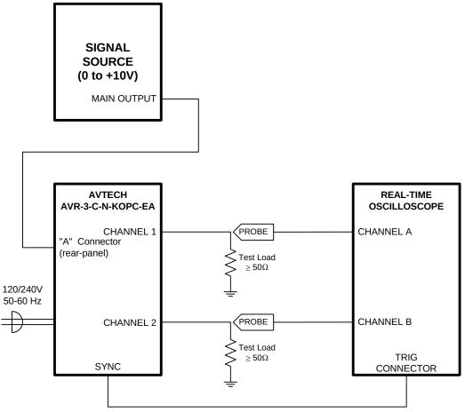
ALL CABLES ARE  $50\Omega$  COAXIAL CABLES.
