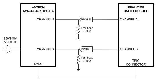
ALL CABLES ARE  $50\Omega$  COAXIAL CABLES.
