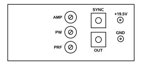
The AMP, PW, and PRF controls may be adjusted using a screwdriver. Rotating the control clockwise increases the affected parameter.
