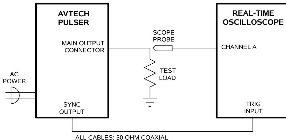
1. Connect a cable from the SYNC OUT connector to the TRIG input of an oscilloscope. Connect a 50W (or higher) 50Ω load to the OUT connector and place the scope probe across this load. The load resistor must have a voltage rating of at least 700V. The power dissipated in the resistor is given by
