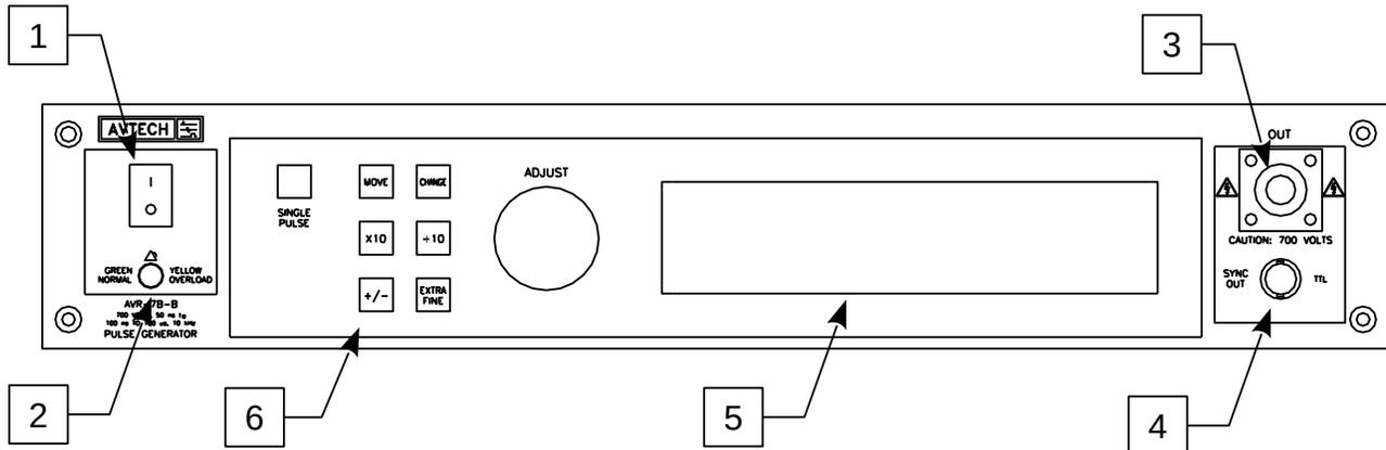
1. POWER Switch. This is the main power switch. When turning the instrument on, there may be a delay of several seconds before the instrument appears to respond.
