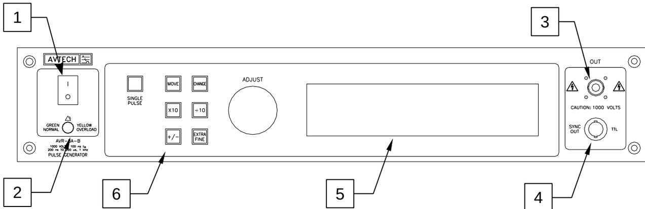
1. **POWER Switch**. This is the main power switch. When turning the instrument on, there may be a delay of several seconds before the instrument appears to respond.
