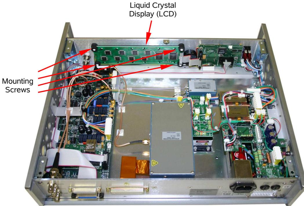
The LCD is an Optrex model C-51849NFJ-SLW-ADN. It is ROHS compliant.
