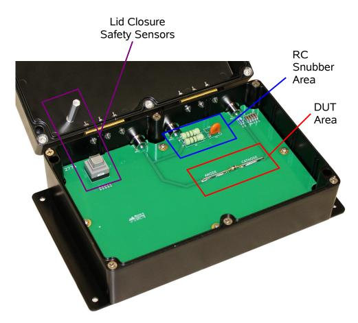
The instrument and the DUT will not be damaged if the diode is installed with the incorrect orientation (i.e., with the anode and cathode reversed). However, incorrect waveforms will be generated.
