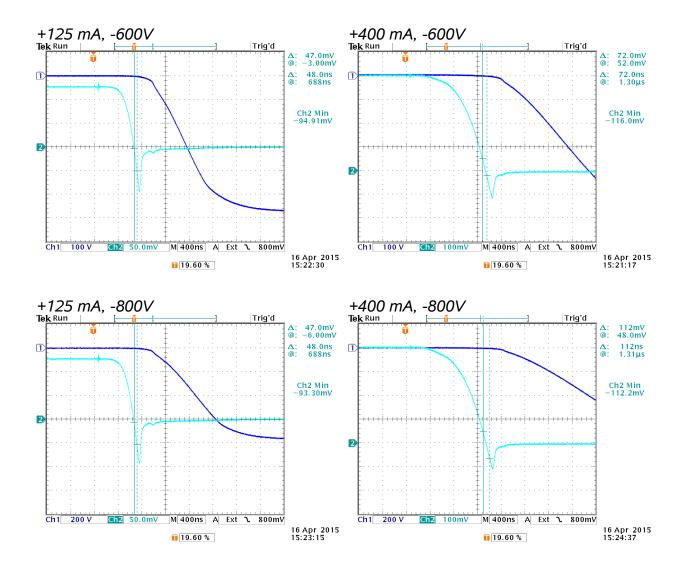
In each photo, the top waveform is the MON output, and the bottom waveform is the OUT waveform (1 mV = 1 mA).
