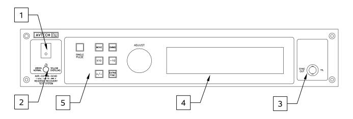
1. <u>POWER Switch</u>. This is the main power switch. When turning the instrument on, there is normally a delay of 5-10 seconds before anything is shown on the main display.
