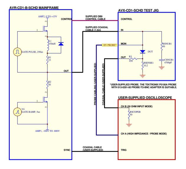
The AVR-CD1-B-SCHD includes an internal trigger source, but it can also be triggered or gated by an external source. A front-panel pushbutton can also be used to trigger the instrument.
