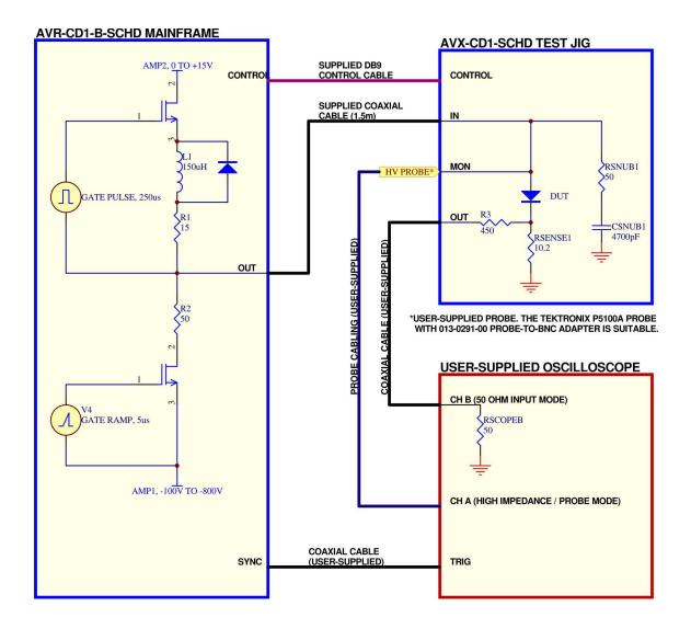
The DUT current is sensed by the resistance in series with the DUT, which consists of RSENSE1 (10.2 $\Omega$ ) in parallel with R3 + RSCOPEB = 500 $\Omega$ , for a total effective series
