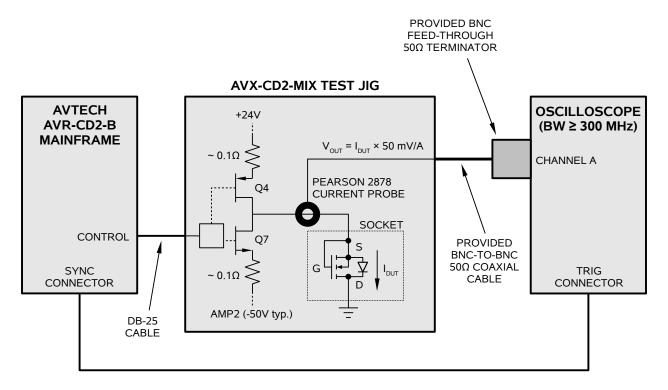
The embedded Pearson 2878 current transformer monitors the current through the DUT, and provides the output signal.
