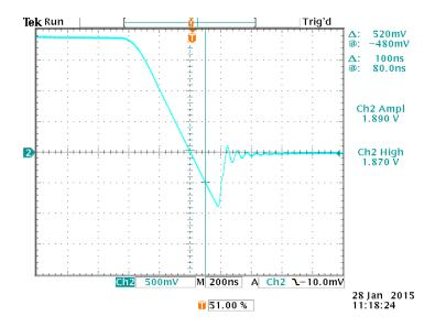
In the waveform above,  $I_F = 1.87 \text{ V} \div 50 \text{ mV/A} = +37.4 \text{A}$ .
