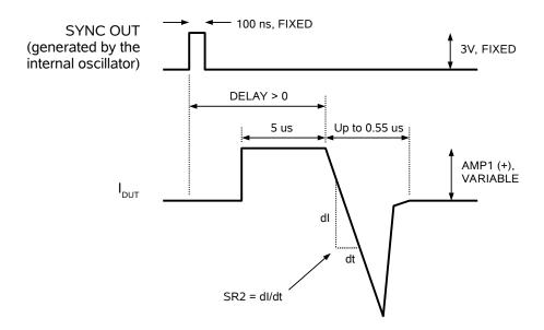
The delay and frequency (when in the internal mode) of the PULSE output can be varied with front panel controls or via the GPIB or RS-232 computer interfaces.
