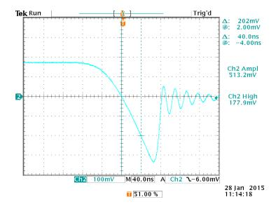
In the waveform above,  $I_F = 177.9 \text{ mV} \div 50 \text{ mV/A} = +3.558\text{A}$ .
