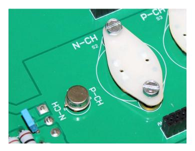
MIL-PRF-19500/556L specifies that the 2N6782 body diode shall be tested with  $I_F$  = +3.5A and dI/dt  $\leq$  100 A/us, and the resulting  $t_{RR}$  shall be less than 180 ns.
