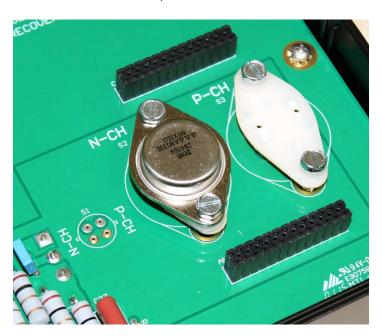
Note that the two screws *must* be tightened and used to provide electrical contact with the drain/case.
