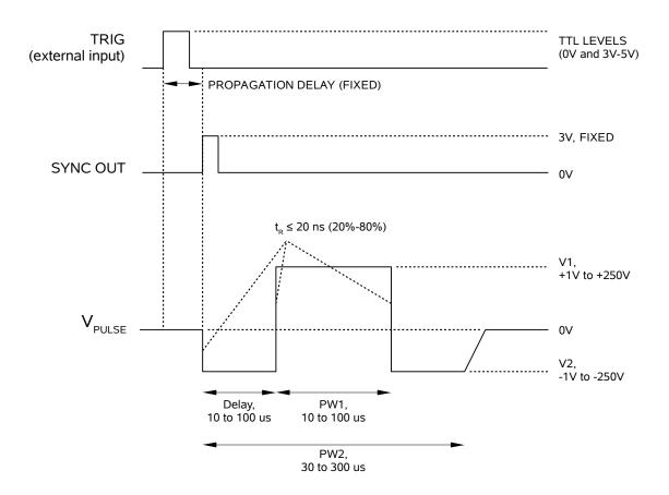
The delay, pulse width, and frequency (when in the internal mode), of the OUT pulse can be varied with front panel controls or via the GPIB or RS-232 computer interfaces.
