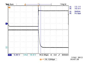
The top waveform shows  $V_{IN}$  swinging from -2V to +10.7V, approximately.
