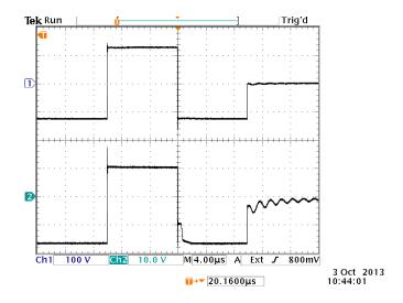
V<sub>MON</sub> shows that the pulser is generating a fast-switching pulse.
