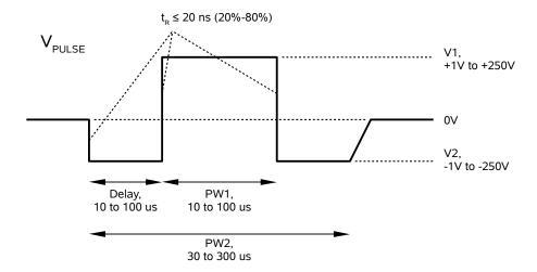
In the waveform shown above, a wide negative pulse (with pulse width PW2 and amplitude -V2) is interrupted by a shorter positive pulse (PW1, +V1). The three highlighted transition have switching times of 20 ns or less. (The final transition to ground is slower).
