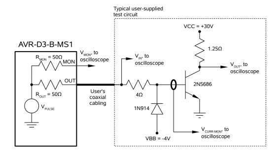
A 50 Ohm output impedance exists between the internal pulse generator circuit and the output connector on the front panel of the instrument.
