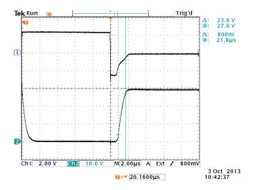
$t_{\text{OFF}}$  is measured as 800 ns. MIL-PRF-19500/464G specifies  $t_{\text{OFF}}$  to be 3.0 us or less, so this particular device meets the test requirements.
