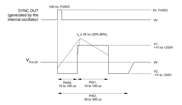
The next figure illustrates the relationship between the signal when an external TTL-level trigger is used:
