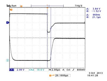
The top waveform shows the output of a current probe on the base ( $V_{\text{CURR-MON}}$ , scaled at 1V/A) swinging from +2.5A to -2.5A, approximately.
