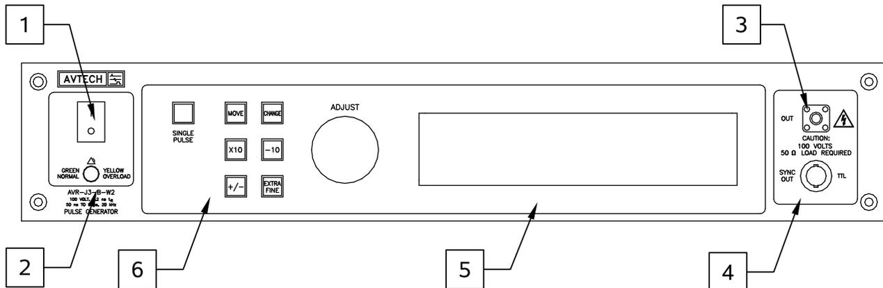
1. POWER Switch. This is the main power switch. When turning the instrument on, there is normally a delay of 10 seconds before anything is shown on the main display, as the internal operating system boots up.
