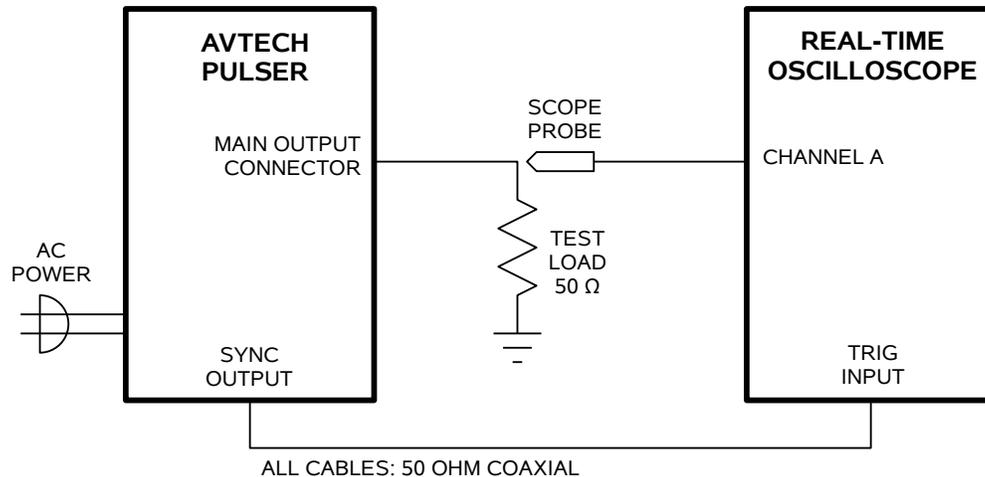
*BASIC TEST ARRANGEMENT, WITH A REAL-TIME OSCILLOSCOPE*
