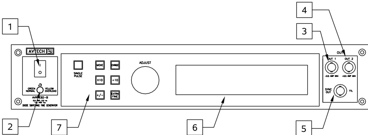
1. POWER Switch. This is the main power switch. When turning the instrument on, there may be a delay of several seconds before the instrument appears to respond.
