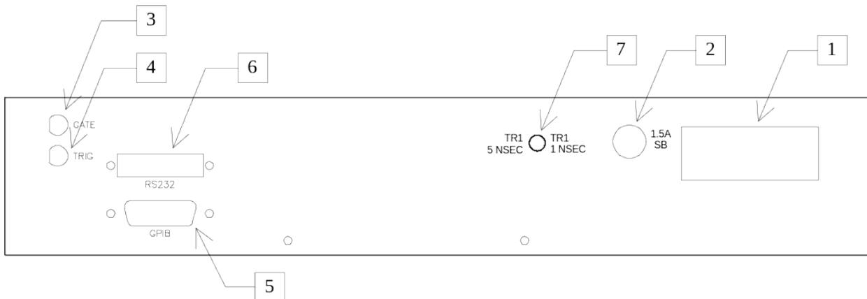
1. **AC POWER INPUT.** A three-pronged recessed male connector is provided on the back panel for AC power connection to the instrument. Also contained in this assembly is a slow-blow fuse and a removable card that can be removed and repositioned to switch between 120V AC in and 240V AC in.
