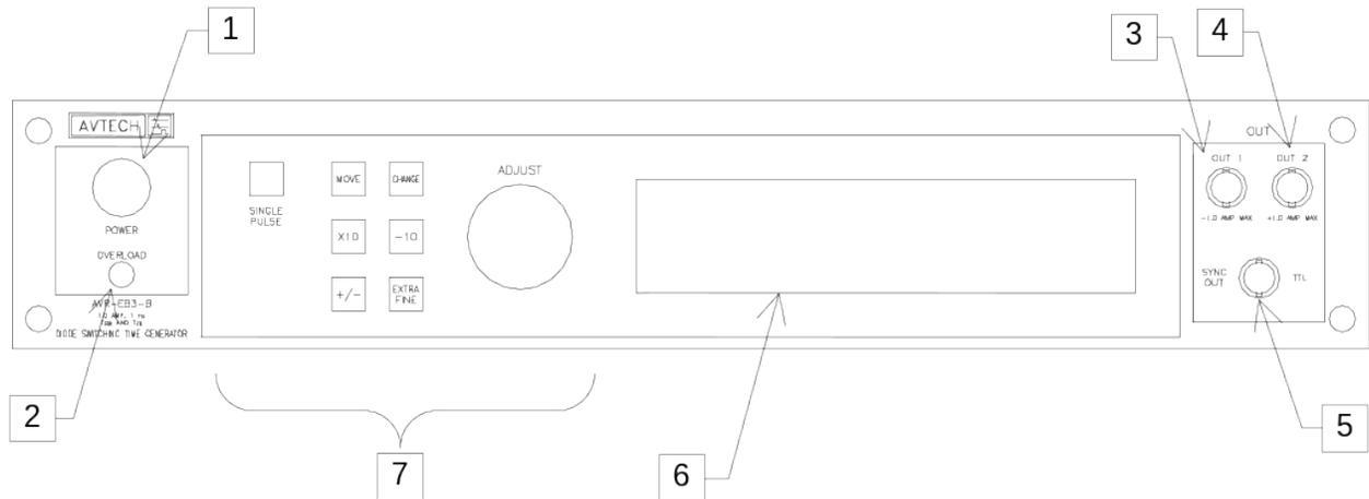
1. **POWER Switch.** The POWER push button switch applies AC prime power to the primaries of the transformer, turning the instrument on. The push button lamp is connected to the internal +15V DC supply.
