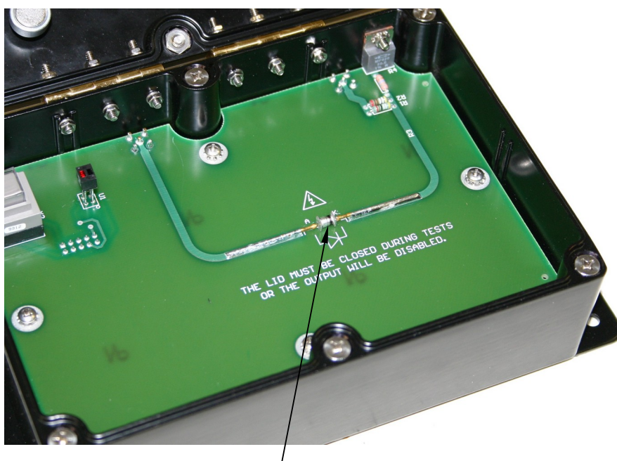
A MELF-packaged Device Under Test (DUT)
