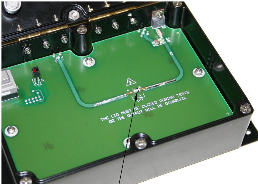
A MELF-packaged Device Under Test (DUT)
