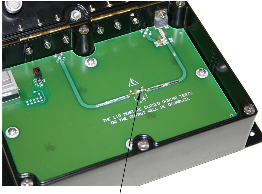
A MELF-packaged Device Under Test (DUT)
