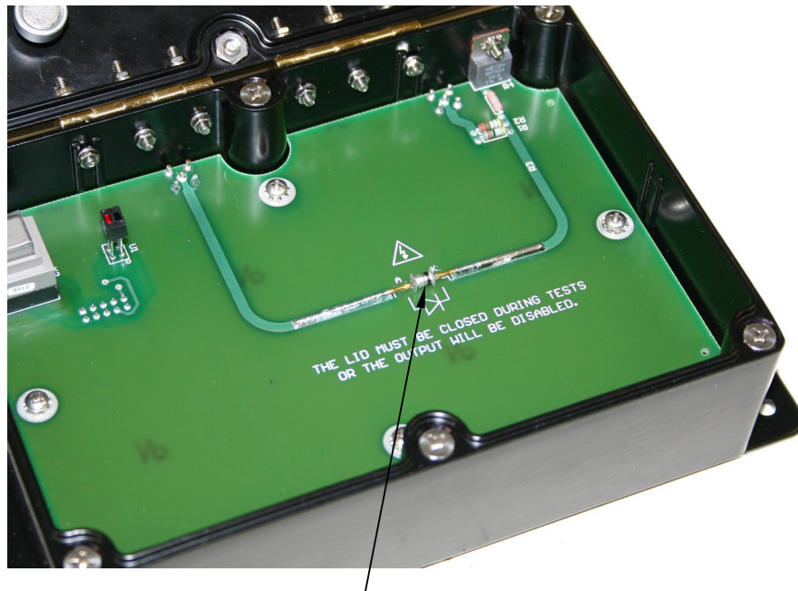
A MELF-packaged Device Under Test (DUT)
