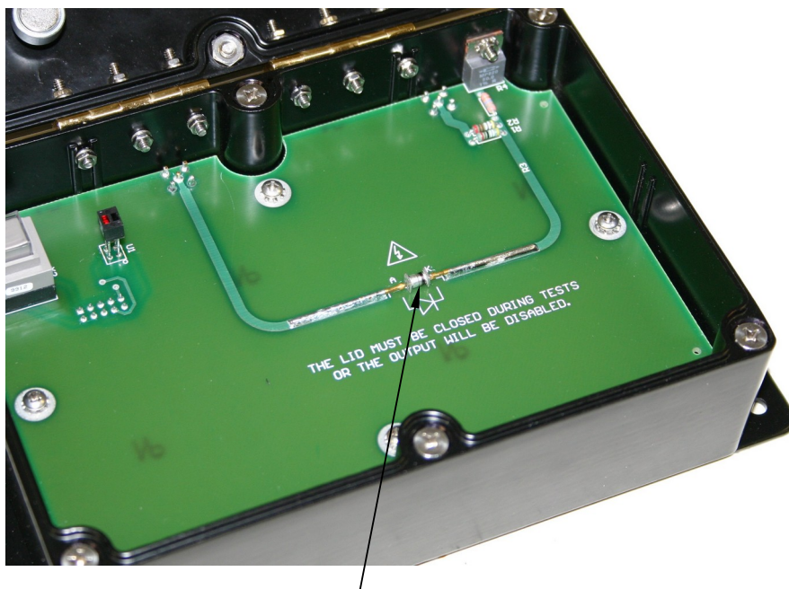
A MELF-packaged Device Under Test (DUT)
