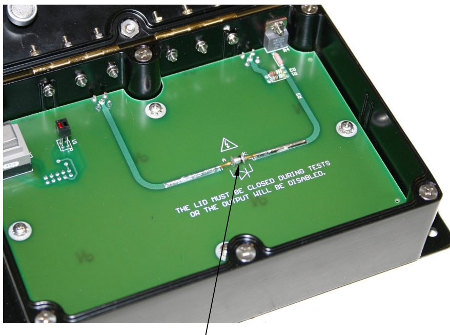
A MELF-packaged Device Under Test (DUT)
