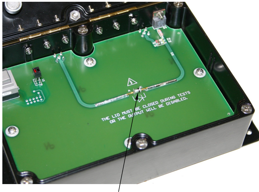
A MELF-packaged Device Under Test (DUT)
