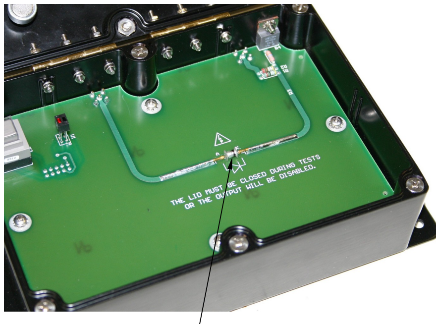
A MELF-packaged Device Under Test (DUT)
