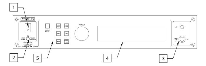
1. <u>POWER Switch</u>. This is the main power switch. When turning the instrument on, there is normally a delay of 10 seconds before anything is shown on the main display, as the internal operating system boots up.
