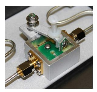
The DUT is inserted into this slot. The anode fits in the wider section of the slot, and the cathode in the narrower section. The anode will contact a section of gold-plated microstrip line, and the cathode will contact a gold-plated ground plane. The aluminum arm must then be positioned over top of the DUT, to apply downward pressure, ensuring that both the anode and cathode contacts the gold areas of the PCB.
