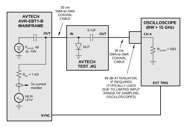
The user may construct their own test jigs using high-bandwidth microstrip construction techniques. The 0.1uF capacitor must be included on the test jig, or a coaxial "DC inner block" may be used instead. The Pasternack PE8210 is an example of a suitable coaxial DC inner block. If the DC block is used, the setup would be modified slightly:
