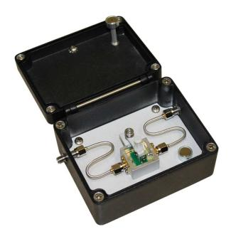
The green PCB in the center of the jig has a slot in its center, which is visible if the spring-loaded aluminum arm is moved out of the way:
