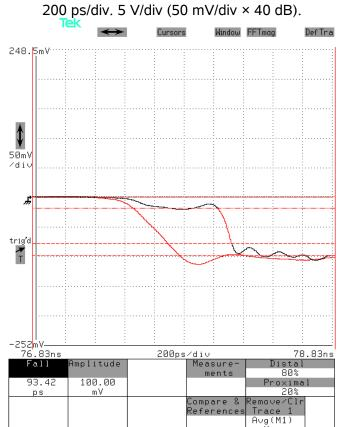
Black = with DUT installed, Red = with DUT removed.
