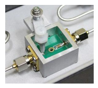
The cathode of the DUT is inserted into this hole. It will make contact with a flexible copper arm on the bottom (ground plane) side of the PCB. The copper arm should move slightly, and hold the cathode end secure. The nylon arm must then be positioned over top of the DUT anode, to apply downward pressure, ensuring that the anode contacts the gold ring around the hole:
