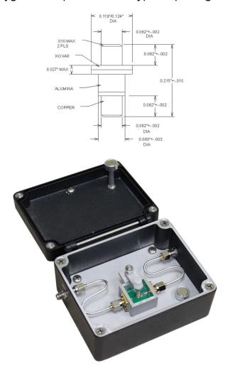
The green PCB in the center of the jig has a hole in its center, which is visible if the spring-loaded nylon arm is moved out of the way:
