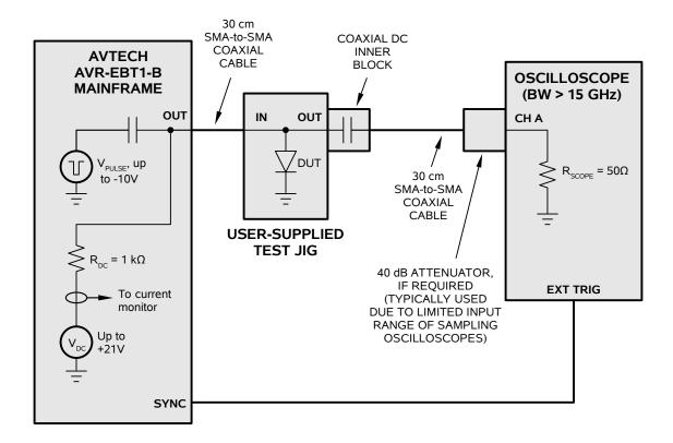
The OUT output on the test jig (or of the DC block, if used) must be connected to the 50 Ohm input of a high-bandwidth (> 15 GHz) user-supplied oscilloscope. The oscilloscope may be used to observe the transition time of the SRD voltage waveform.
