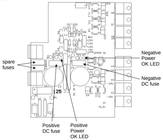
The positive fuse and one of the spare fuses on this circuit board are 2A slow-blow fuses, Littlefuse part number R452002. (This fuse can be ordered from Digikey, www.digikey.com. The Digikey part number is F1345CT-ND). The negative fuse and the second spare fuse are 0.5A slow-blow fuses (Littlefuse R452.500, Digikey part number F1341CT-ND).
