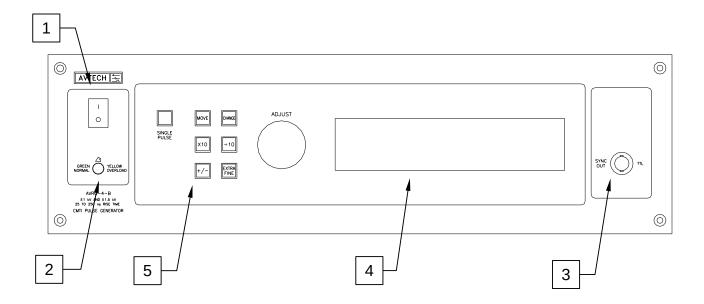
1. <u>POWER Switch</u>. This is the main power switch. When turning the instrument on, there is normally a delay of 10 seconds before anything is shown on the main display, as the internal operating system boots up.
