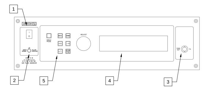
1. <u>POWER Switch</u>. This is the main power switch. When turning the instrument on, there is normally a delay of 5-10 seconds before anything is shown on the main display.
