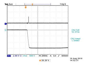
Removing the pin socket for pin 7, thus reducing stray capacitance, is enough to almost double the observed dV/dt rating.
