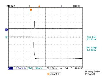
Removing the pin socket for pin 7, thus reducing stray capacitance, is enough to almost double the observed dV/dt rating.
