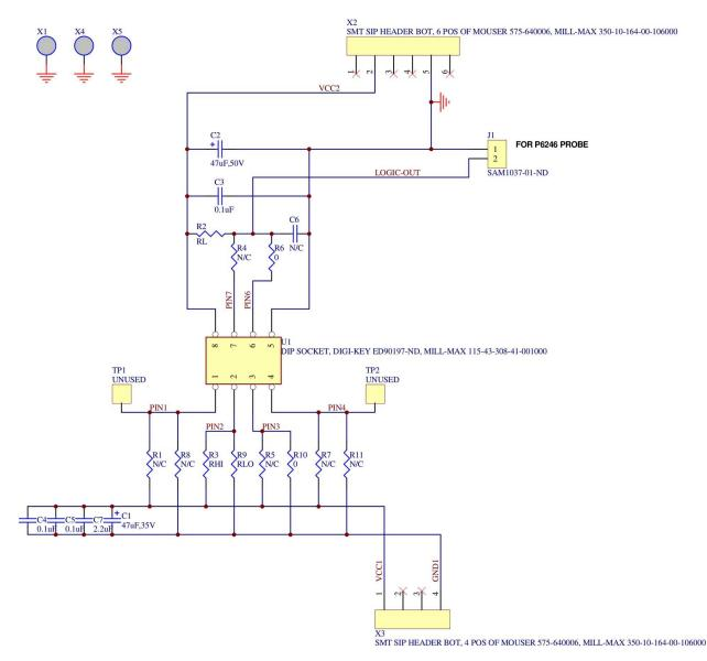
Any of pins 1 to 4 may be connected directly to VCC1 or GND1 use a zero-ohm jumper in the appropriate location. For example, a voltage-powered device would normally install R1=0 (to connect VCC1 to pin 1) and R11=0 (to connect GND1 to pin 4). The logic inputs (on pins 2 and 3) would then be connected to VCC1 or GND1 as desired using R3, R9, R5, and/or R10.
