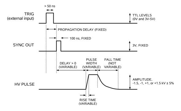
As before, if the delay is negative, the order of the SYNC and OUT pulses is reversed.
