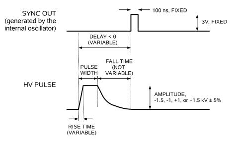
The next figure illustrates the relationship between the signals when an external TTLlevel trigger is used:
