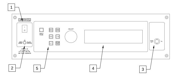
1. <u>POWER Switch</u>. This is the main power switch. When turning the instrument on, there is normally a delay of 5-10 seconds before anything is shown on the main display.
