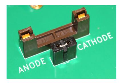
The two sockets are wired in parallel. Only one DUT may be installed at a time, or the resulting waveforms will be incorrect.
