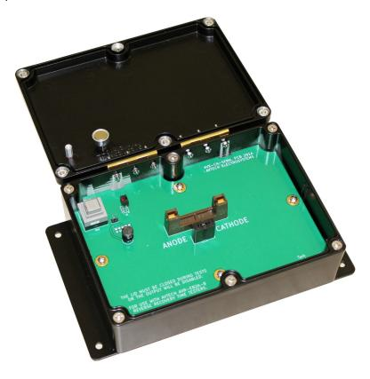
Install a diode in one of the two sockets. An example of an axial DO-41 diode installed is shown below:
