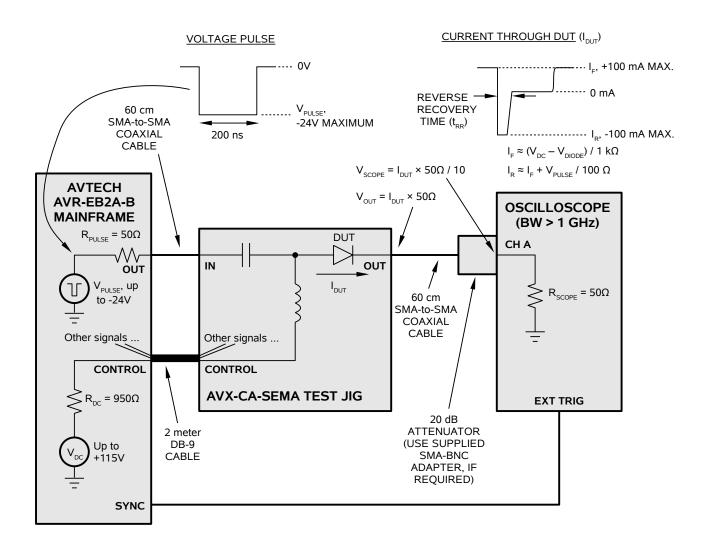
The OUT output on the test jig must be connected (using the 60 cm SMA-to-SMA cable and 20 dB attenuator supplied with the AVR-EB2A-B) to the 50 Ohm input of a high-bandwidth (> 1 GHz) user-supplied oscilloscope. The voltage on the output is proportional to the current through the DUT. By observing the current waveform through
