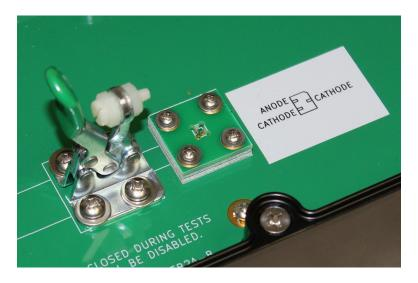
Using tweezers, position a DUT in the cavity of the raised circuit boards. The DUT will rest on three spring pins, one contacting each DUT pad:
