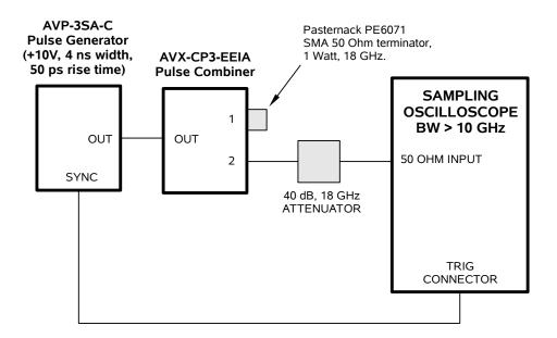
The output signal measured at the oscilloscope will have a rise time of < 500 ps (measured 20%-80%).
