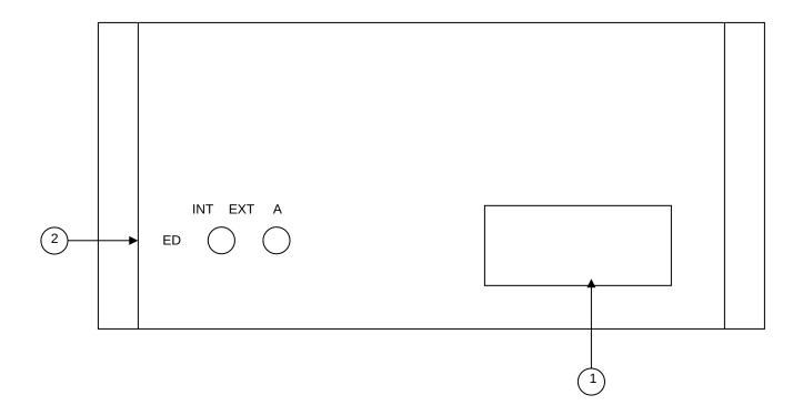
(1) <u>FUSED CONNECTOR, VOLTAGE SELECTOR</u>. The detachable power cord is connected at this point. In addition, the removable cord is adjusted to select the desired input operating voltage. The unit also contains the main power fuse.
