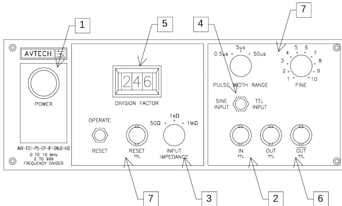
1. **POWER Switch.** The POWER push button switch applies AC prime power to the primaries of the transformer, turning the instrument on. The push button lamp (#382 type) is connected to the +15V DC supply.
