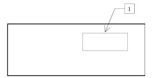
1.<u>AC POWER INPUT</u>. A three-pronged recessed male connector is provided on the back panel for AC power connection to the instrument. Also contained in this assembly is a slow-blow fuse and a removable card that can be removed and repositioned to switch between 120V AC in and 240V AC in.
