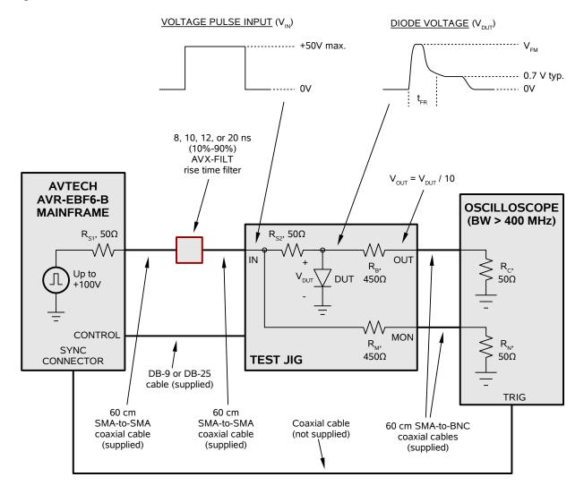
The AVR-EBF6-B mainframe connects to the rise time filter using a 60 cm length of SMA-to-SMA coaxial cable.
