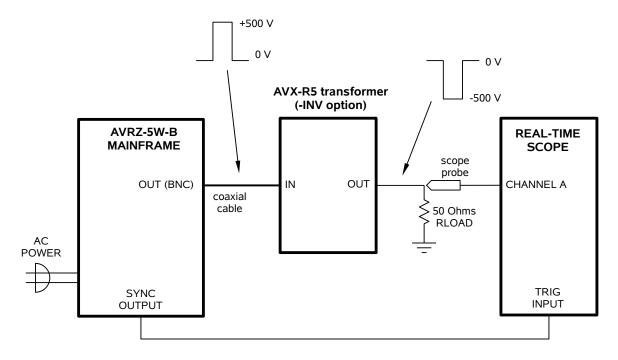
The transformer is capable of operating up to the maximum rated pulse width of the AVRZ-5W-B and AVRZ-5A-B (10 us). The transformer may introduce slight rounding and ringing to the output waveform, and it may degrade rise and fall times by several nanoseconds. A typical waveform photo is shown below:
