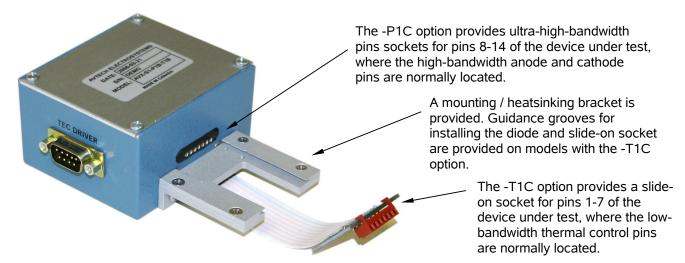
The diode is first installed by sliding pins 8-14 into the "P1C" pin sockets, as shown below:
