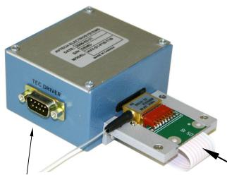
Gently slide the low-bandwidth slide-on socket onto the matching pins of the device under test. The slideon socket is connected to the output module using a short length of flexible ribbon cable. The thermoelectric cooler and thermistor pins are made accessible to the user through the "TEC DRIVER" DB-9 connector, which will mate to cables from common third-party TEC controllers.
