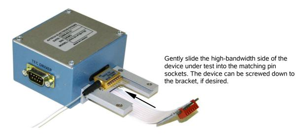
If present, the T1C slide-on socket assembly can then be slid onto pins 1-7, as shown below:
