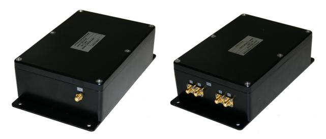
The one input and four output SMA connectors are located on opposite ends of the module, as shown above.
