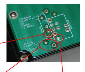
This spring pin must contact the underside of the case. It provides the cathode connection.
