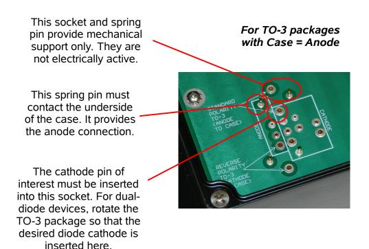
If the case is connected to the cathode, and the pin(s) are used for the anode, the arrangement shown below must be used:
