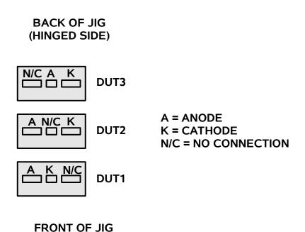
This test jig can be used as a replacement or an alternative for the test jigs originally supplied with the Avtech AVR-EBF6-B units.
