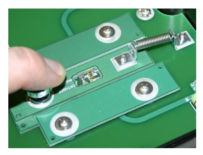
The DUT is then placed in the area immediately in front of the two fixed probe points, as shown in the photo above. Then slowly release the chrome knob, allowing the spring-loaded PCB to push the DUT into position against the two probe points, as shown below. The PCB silk-screening shows the proper device positioning.
