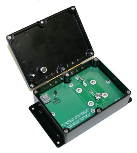
The DUT is installed by pulling back on the chrome knob, as shown below:
