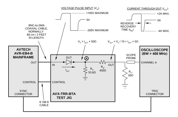
$\triangle$  A 50 Ohm resistance (R<sub>C</sub> in the diagram above) must be connected to ground on the output. This can be a discrete resistor, a feed-through terminator, or the input impedance of an oscilloscope. If a high-speed sampling oscilloscope is used, the input should be protected by adding attenuator on the input.
