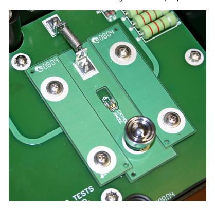
The anode pad must contact the left probe point, and the cathode pin must contact the right probe point.
