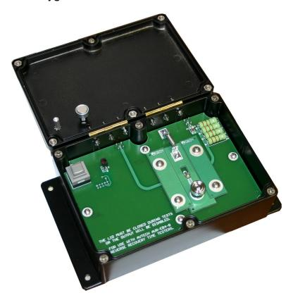
The DUT is installed by pulling back on the chrome knob, as shown below:
