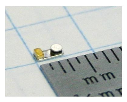
This test jig can be used as a replacement or an alternative for the test jigs originally supplied with the Avtech AVR-EB4-B units.
