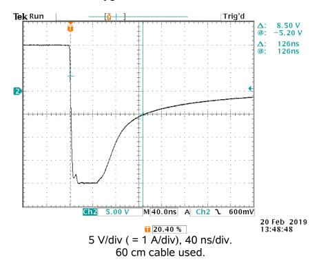
The above waveform shows the transition from a forward current of +2A to a reverse current of -4A. The reverse transient lasts for approximately 126 ns under these conditions (measured at the 25% reverse current point).
