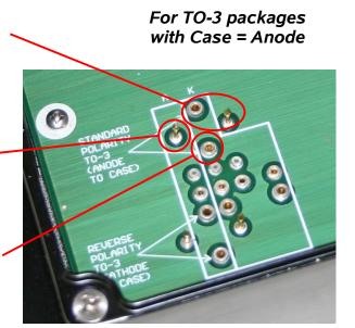
If the case is connected to the cathode, and the pin(s) are used for the anode, the arrangement shown below must be used:
