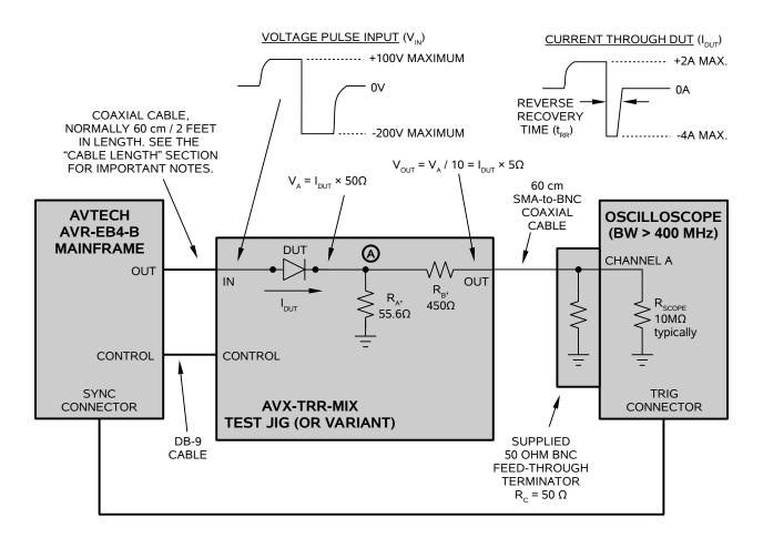
A 50 Ohm resistance (R<sub>C</sub> in the diagram above) must be connected to ground on the output. This can be a discrete resistor, a feed-through terminator, or the input impedance of an oscilloscope. If a high-speed sampling oscilloscope is used, the input should be protected by adding attenuator on the input.
