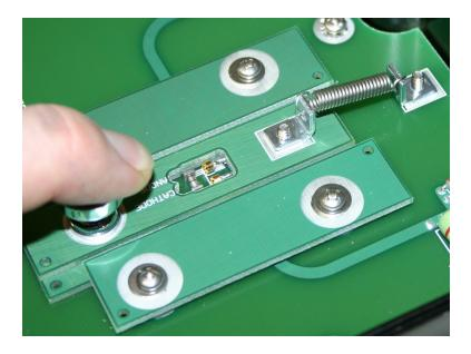
The DUT is then placed in the area immediately in front of the two fixed probe points, as shown in the photo above. Then slowly release the chrome knob, allowing the spring-loaded PCB to push the DUT into position against the two probe points, as shown below. The PCB silk-screening shows the proper device positioning.
