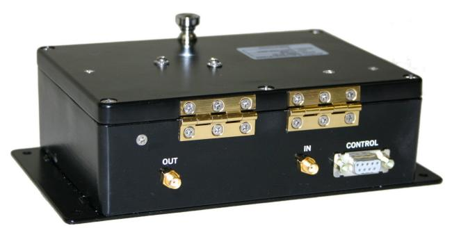
The IN, OUT, and CONTROL connectors are on the rear of the jig, below the hinges:
