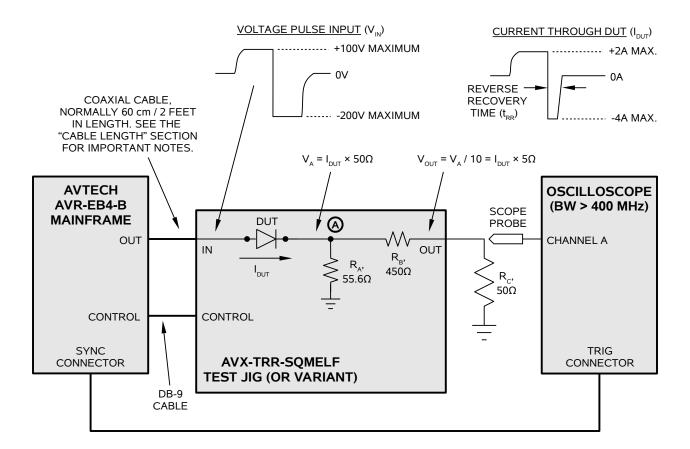
$\triangle$  A 50 Ohm resistance (R<sub>C</sub> in the diagram above) must be connected to ground on the output. This can be a discrete resistor, a feed-through terminator, or the input impedance of an oscilloscope. If a high-speed sampling oscilloscope is used, the input should be protected by adding attenuator on the input.
