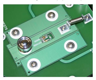
The anode pad must contact the left probe point, and the cathode pin must contact the right probe point.
